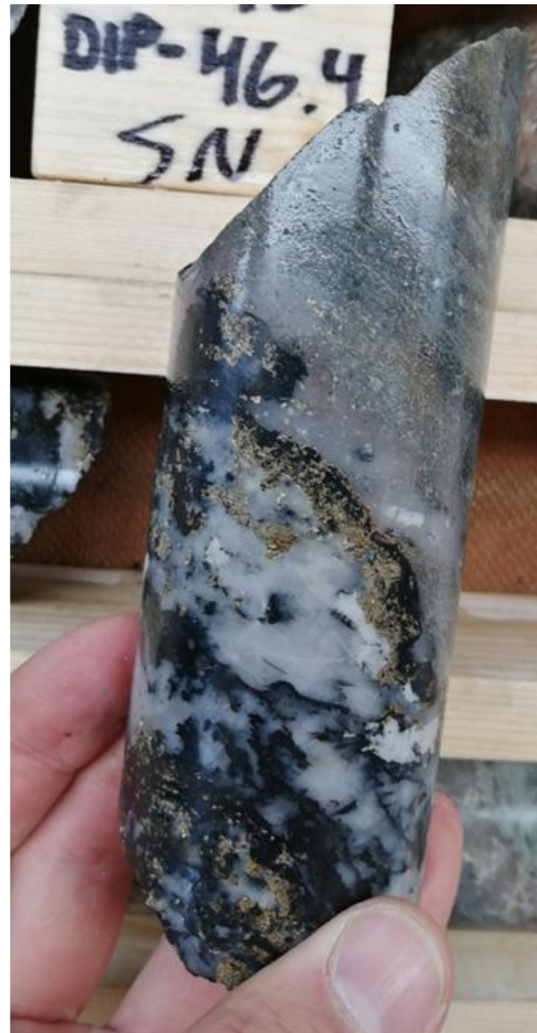
Drill hole 21MJ001. Left: Mineralized quartz-carbonate-tourmaline pyrite veins. Right: Visible Gold
