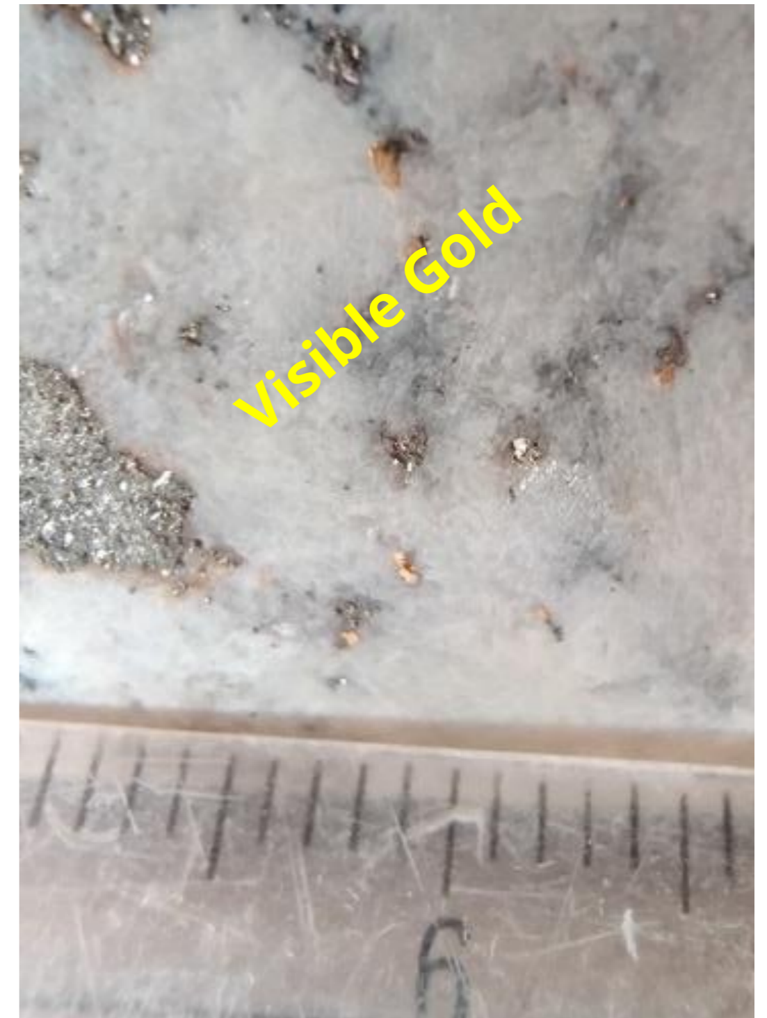
Drill hole 21MJ001. Left: Mineralized quartz-carbonate-tourmaline pyrite veins. Right: Visible Gold
