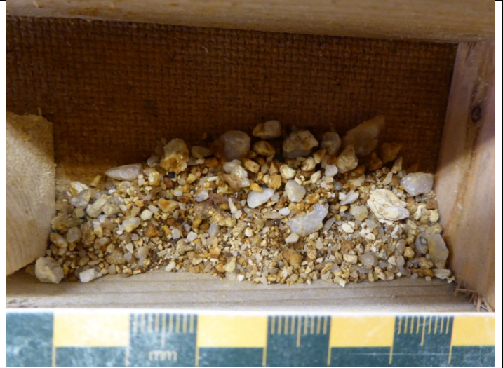
D. Hole MJ-4 (25.7 m). This is a close-up within the previous photo, showing a little fine material left unsampled: vein quartz and goethitic rubble (fault? shear?). This sample interval (25.0-26.0 m) reported 7.25 g/t Au.
