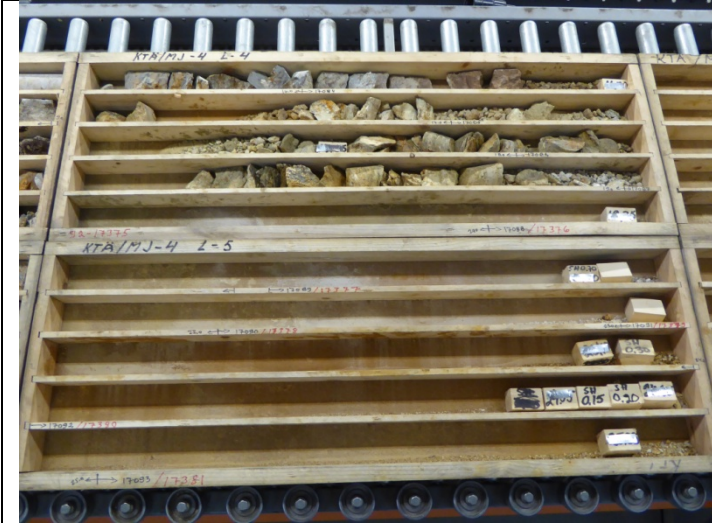
C. Hole MJ-4. Core has been entirely sampled from Au-bearing intervals (19.0-25.8 m in this photo).
