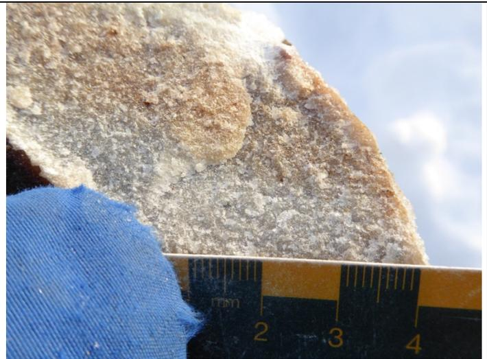
B. Quartzite near collar of hole KOT-2. Faint greenish cast may be due to weak fuchsite alteration.
