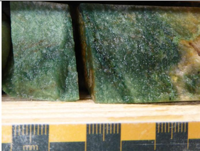
A. Hole KOT-2 (16.7 m; 0.1 ppm Au). Fuchsite-altered quartzite.
